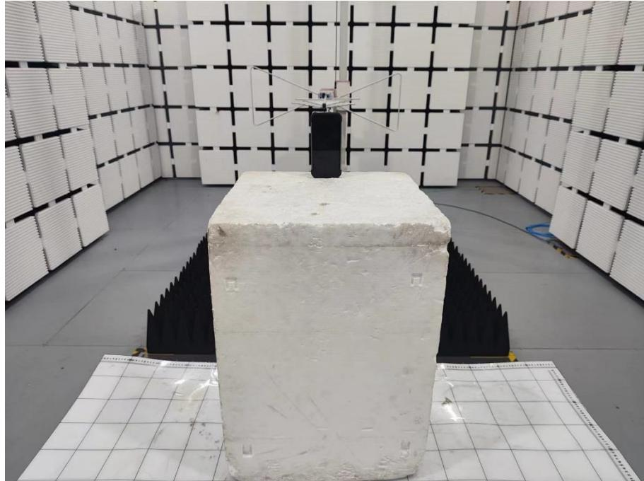
**Set-up for Transmitter & Receiver Spurious Emissions, Above 1GHz**
