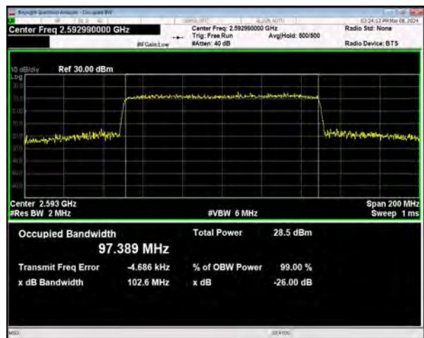
n41 SCS=30kHz CP_16QAM BW=100MHz Channel=518598 RB=273@0
