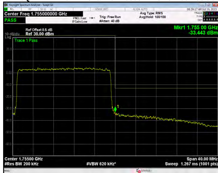
Band4 16QAM BW=3MHz Channel=19965 RB Size=15 Position=#0
