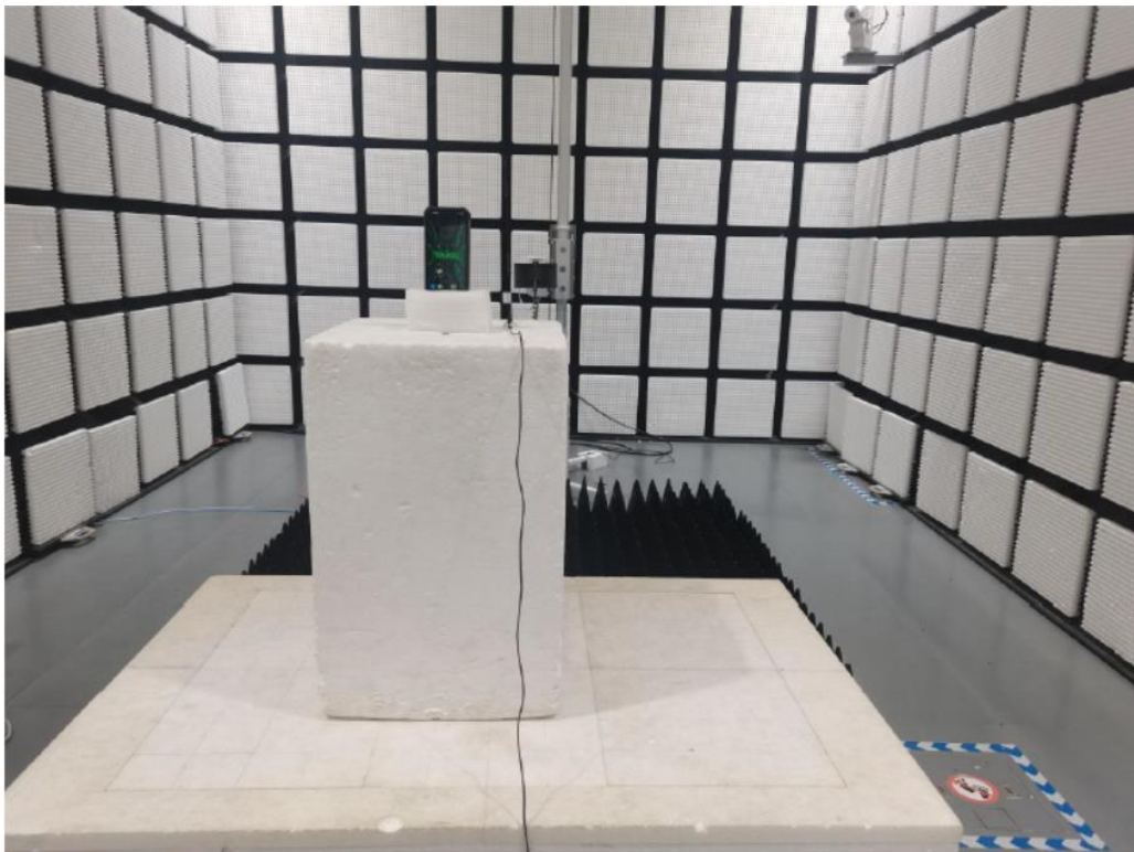
Set-up for Radiated Spurious Emission, Above 1GHz
