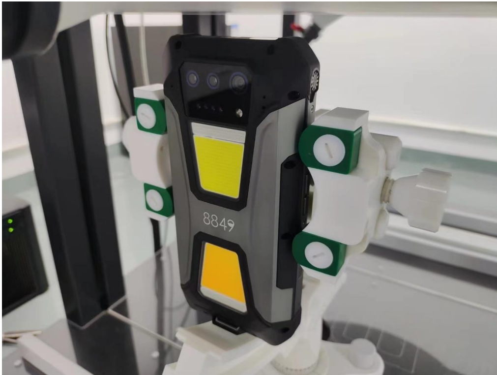
Body Top side (separation distance is 10mm)
