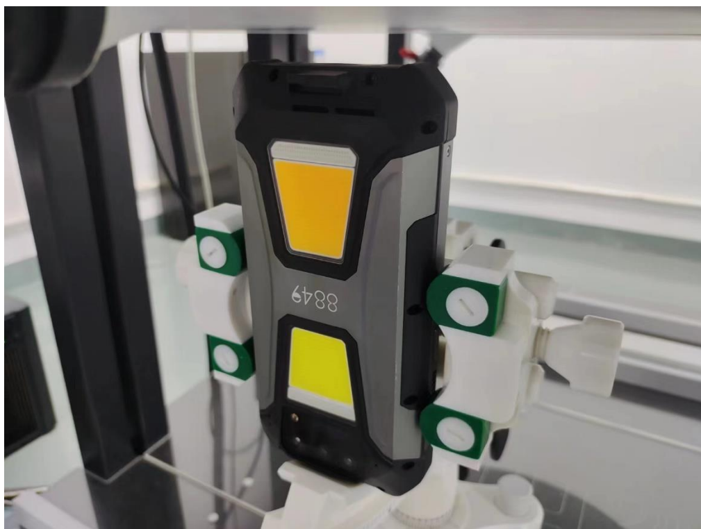
Body Bottom side (separation distance is 10mm)
