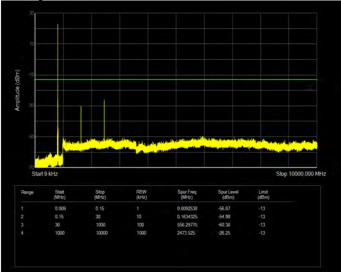
Band5 QPSK BW=5MHz Channel=20525 RB Size=1 Position=#0
