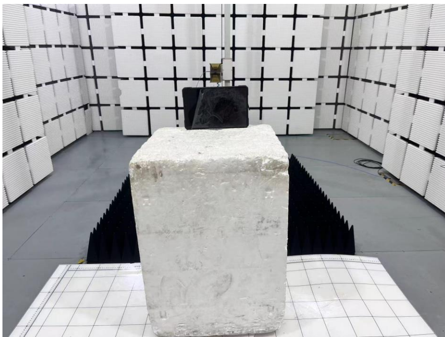
Set-up for Radiated Spurious Emission, Above 1GHz
