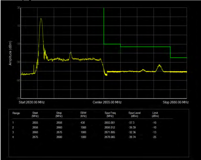
Band41(2555-2655) QPSK BW=5MHz Channel=40265 RB Size=1 Position=#0 Extended
