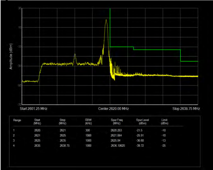
Band38 QPSK BW=15MHz Channel=38175 RB Size=75 Position=#0 Extended
