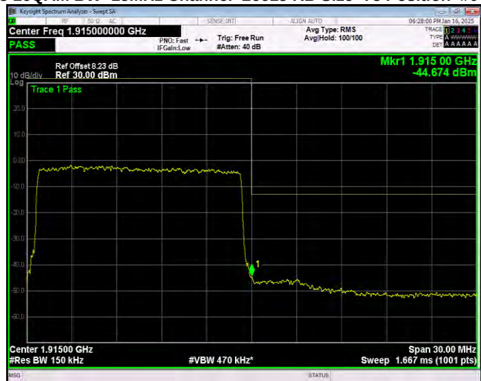
Band25 16QAM BW=15MHz Channel=26615 RB Size=75 Position=#0 Normal
