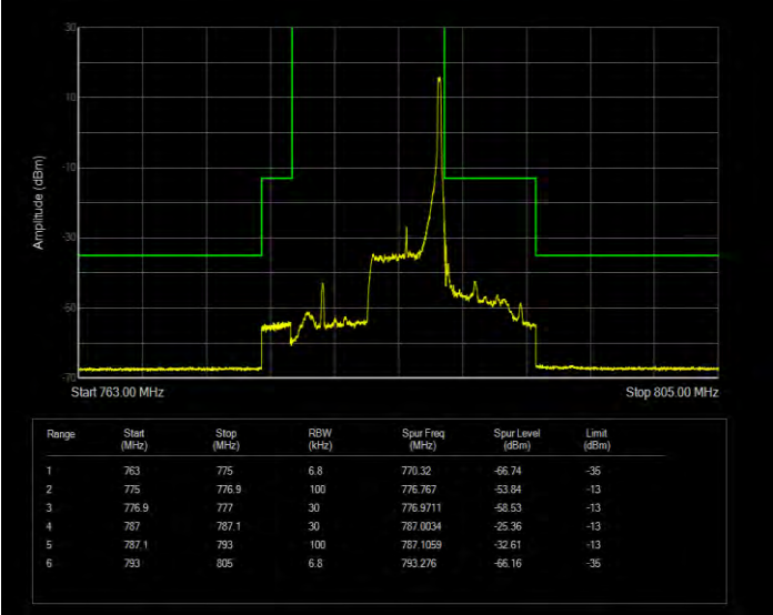
Band13 16QAM BW=5MHz Channel=23255 RB Size=25 Position=#0 Extended
