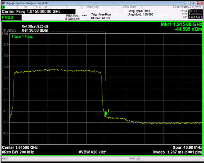
Band25 16QAM BW=20MHz Channel=26590 RB Size=100 Position=#0 Normal
