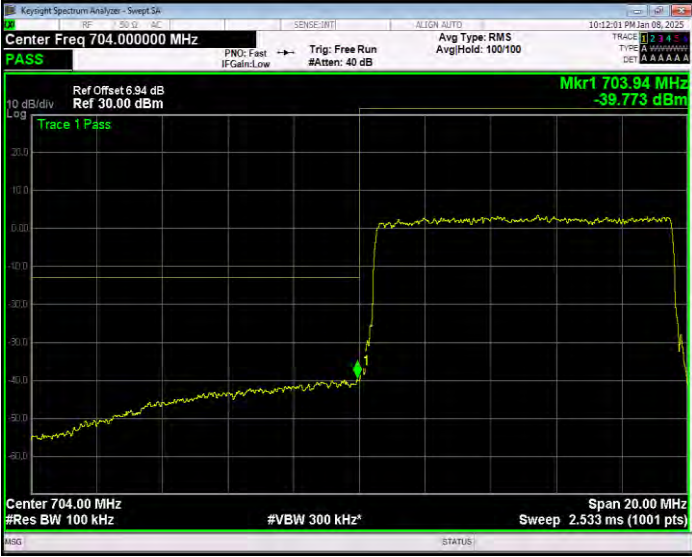
Band17 16QAM BW=10MHz Channel=23780 RB Size=50 Position=#0 Normal
