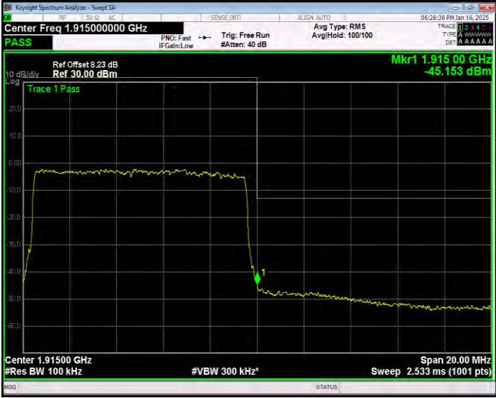
Band25 16QAM BW=10MHz Channel=26640 RB Size=50 Position=#0 Normal
