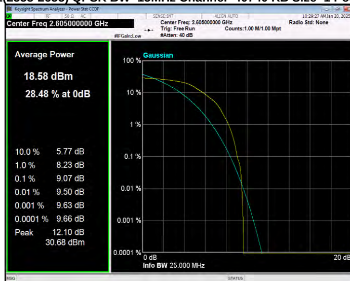
Band41(2555-2655) QPSK BW=15MHz Channel=40740 RB Size=1 Position=#0
