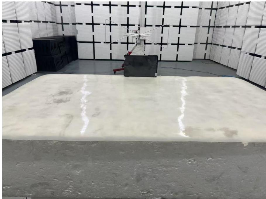
**Set-up for Transmitter & Receiver Spurious Emissions, Above 1GHz**
