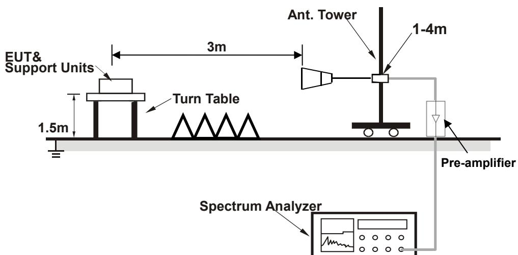
**For radiated test above 18GHz**
