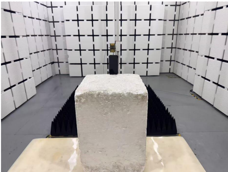
Set-up for Radiated Spurious Emission, Above 1GHz
