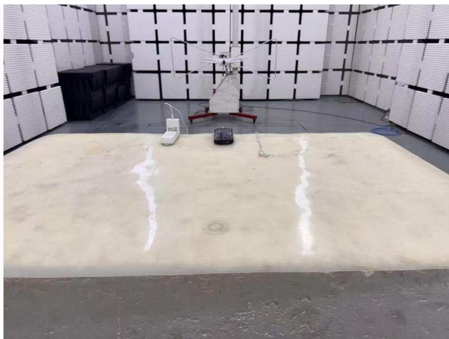
**Set-up for Radiated Emission (RE), Above 1GHz**
