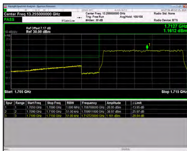
n66 SCS=15kHz DFT_256QAM BW=5MHz LowChannel=342500 RB=25@0
