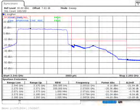
n7 SCS=15kHz DFT_BPSK BW=20MHz HighChannel=512000 RB=100@0
