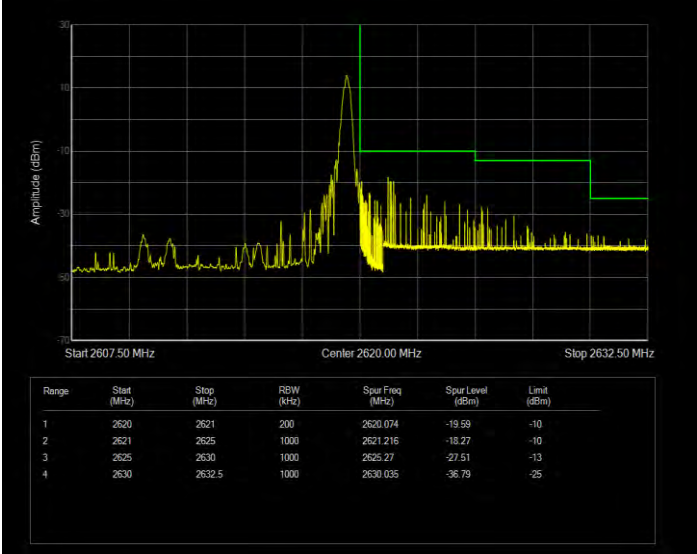
Band38 16QAM BW=10MHz Channel=38200 RB Size=50 Position=#0 Extended
