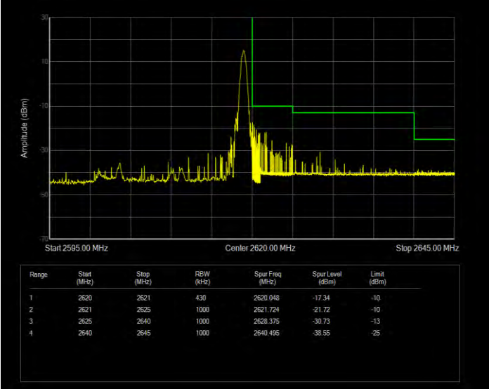
Band38 16QAM BW=20MHz Channel=38150 RB Size=100 Position=#0 Extended
