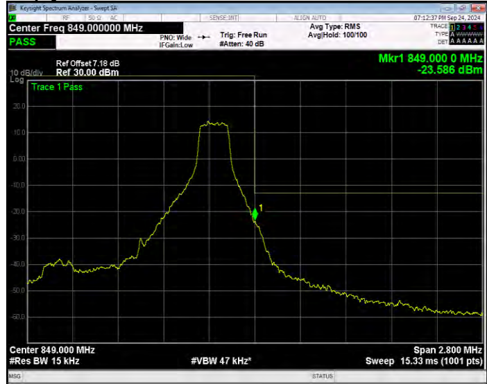
Band26(824-849) QPSK BW=1.4MHz Channel=27033 RB Size=6 Position=#0 Extended
