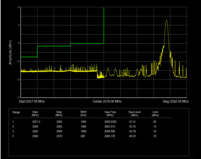
Band38 16QAM BW=10MHz Channel=37800 RB Size=50 Position=#0 Extended
