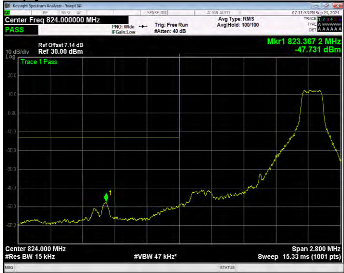
Band26(824-849) QPSK BW=1.4MHz Channel=26797 RB Size=6 Position=#0 Extended
