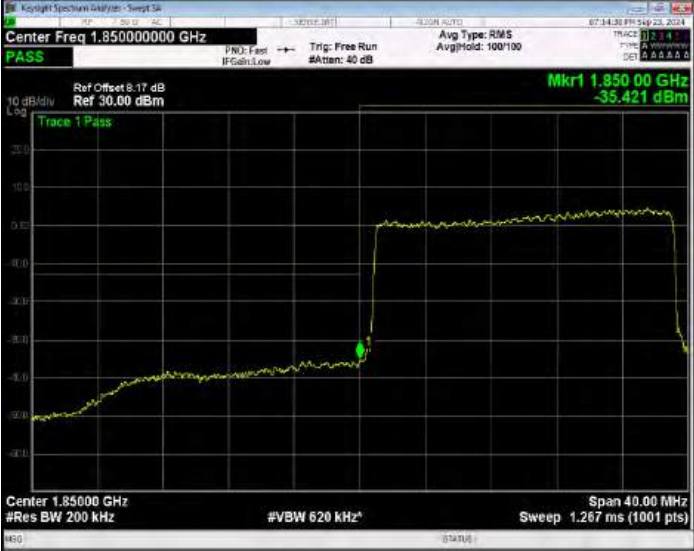
Band2 QPSK BW=20MHz Channel=18700 RB Size=100 Position=#0 Normal
