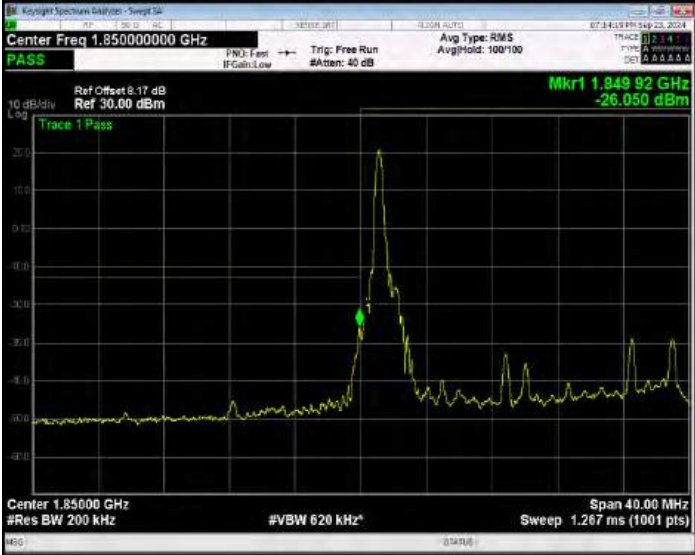
Band2 QPSK BW=20MHz Channel=18700 RB Size=1 Position=#Max Extended
