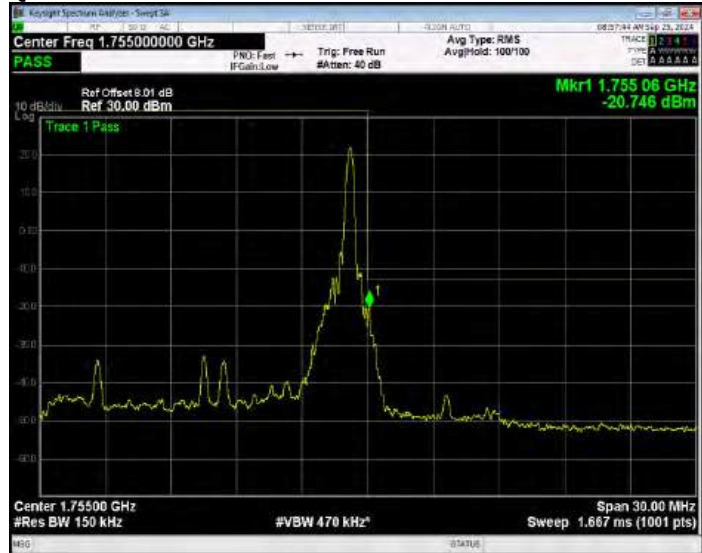
Band4 QPSK BW=15MHz Channel=20325 RB Size=75 Position=#0 Normal
