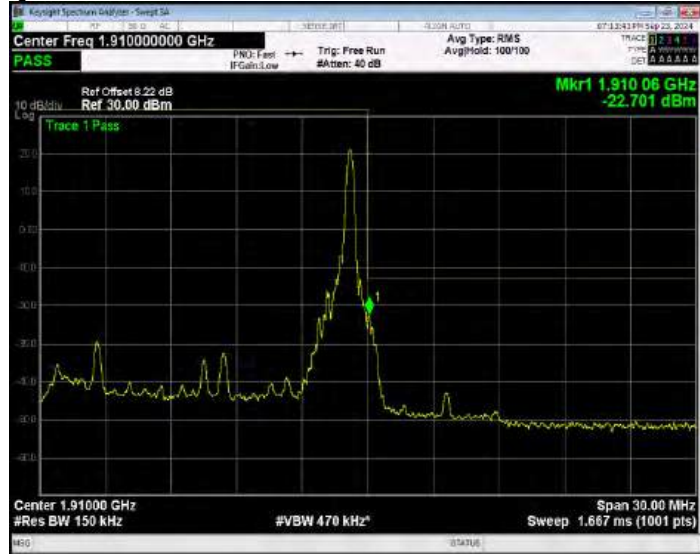
Band2 QPSK BW=15MHz Channel=19125 RB Size=75 Position=#0 Extended
