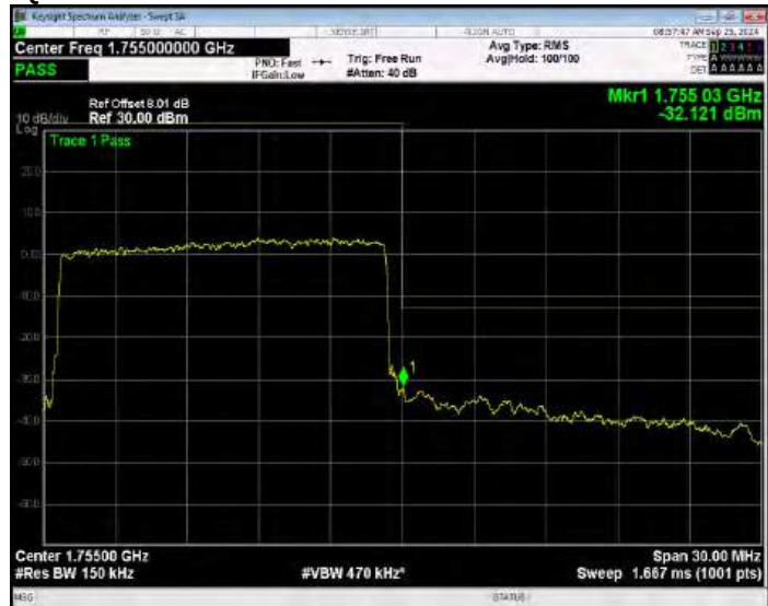
Band4 QPSK BW=15MHz Channel=20325 RB Size=75 Position=#0 Normal
