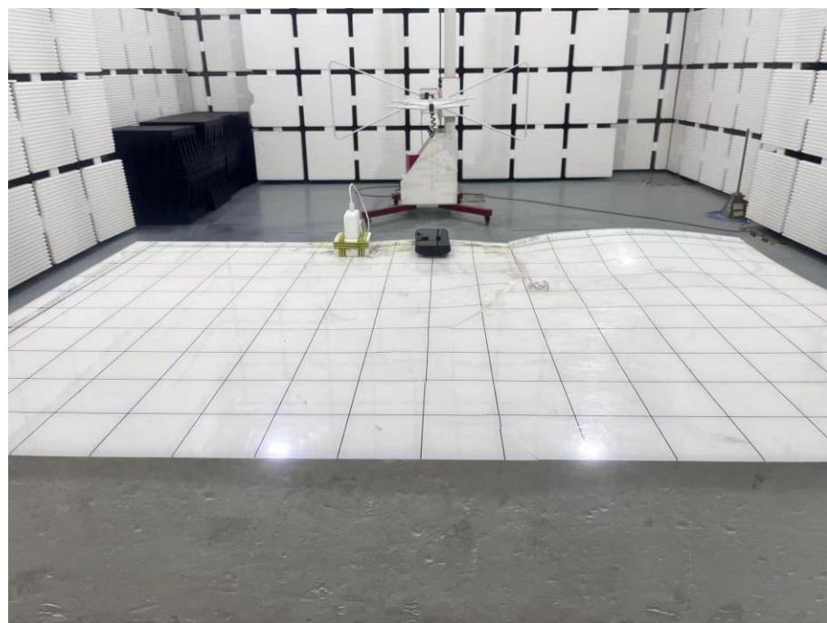
**Set-up for Radiated Emission (RE), Above 1GHz**
