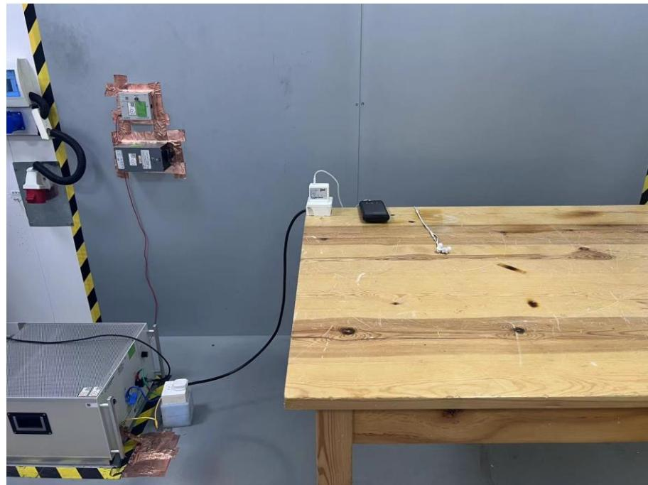
**Set-up for Radiated Emission (RE), Below 1GHz**
