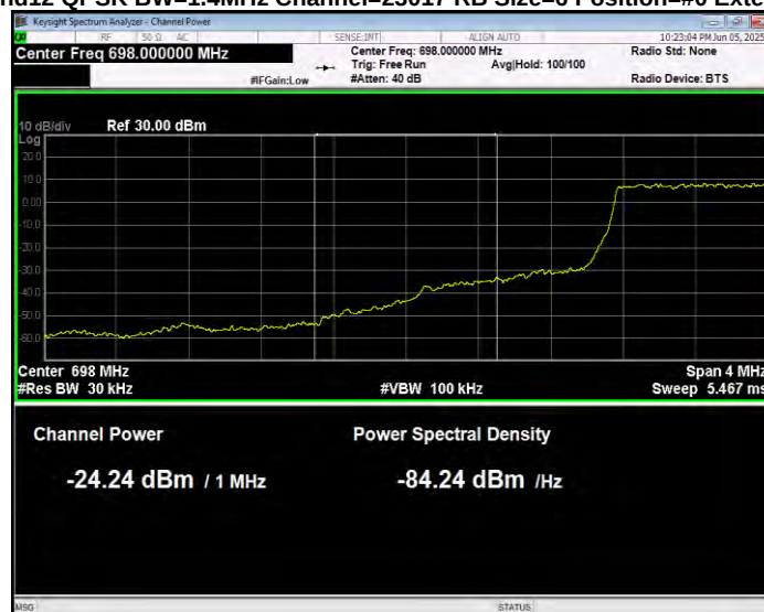
Band12 QPSK BW=1.4MHz Channel=23017 RB Size=6 Position=#0 Normal
