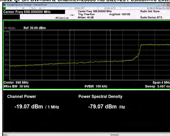
Band12 QPSK BW=5MHz Channel=23035 RB Size=25 Position=#0 Normal
