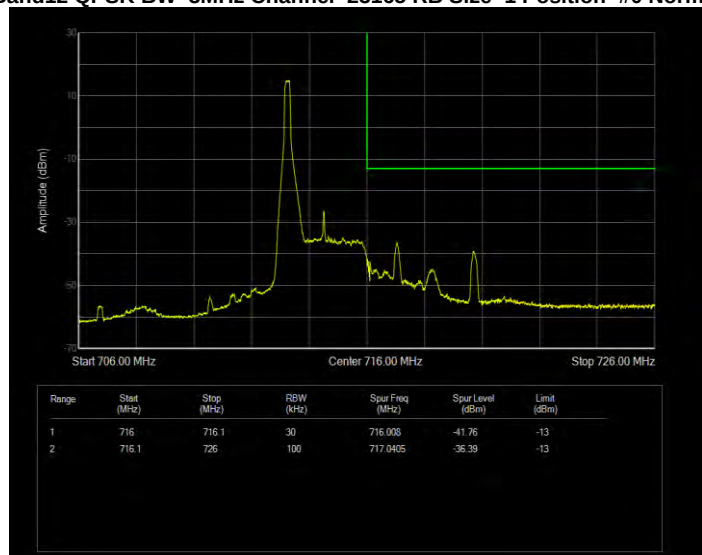
Band12 QPSK BW=3MHz Channel=23165 RB Size=1 Position=#Max Extended
