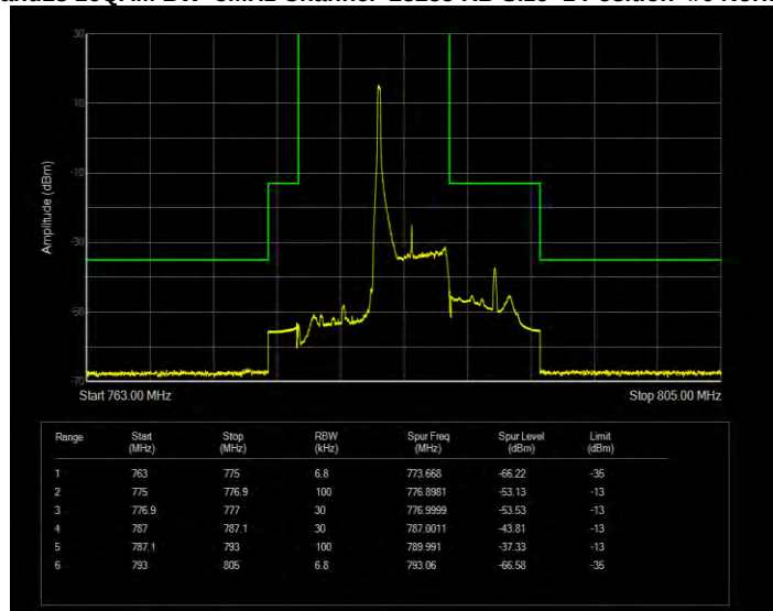
Band13 16QAM BW=5MHz Channel=23255 RB Size=1 Position=#Max Extended
