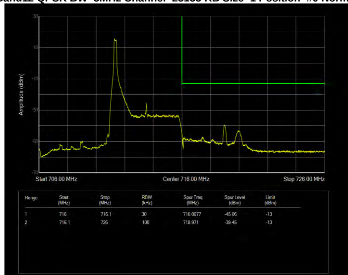
Band12 QPSK BW=5MHz Channel=23155 RB Size=1 Position=#Max Extended
