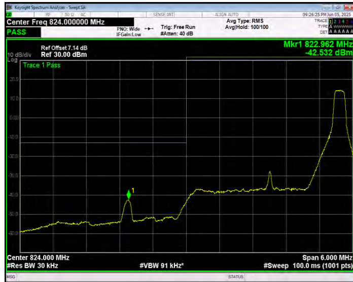
Band5 16QAM BW=3MHz Channel=20415 RB Size=15 Position=#0 Extended
