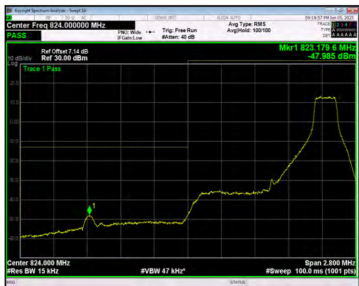
Band5 QPSK BW=1.4MHz Channel=20407 RB Size=6 Position=#0 Extended
