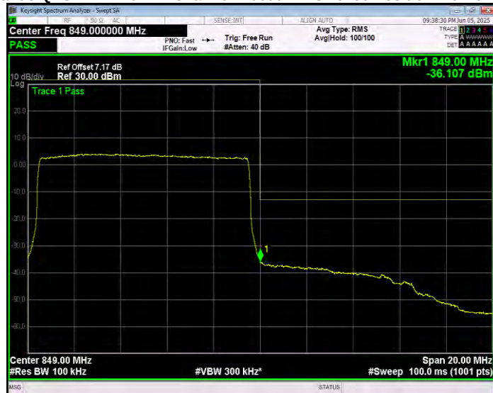
Band5 QPSK BW=3MHz Channel=20415 RB Size=1 Position=#0 Extended
