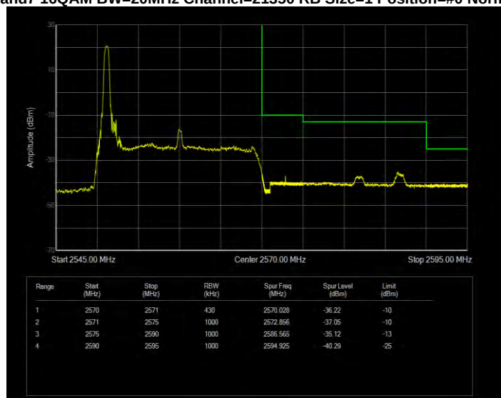
Band7 16QAM BW=20MHz Channel=21350 RB Size=1 Position=#Max Extended
