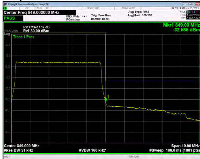
Band7 16QAM BW=10MHz Channel=20800 RB Size=1 Position=#0 Extended
