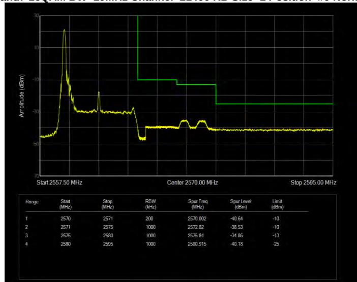
Band7 16QAM BW=10MHz Channel=21400 RB Size=1 Position=#Max Extended
