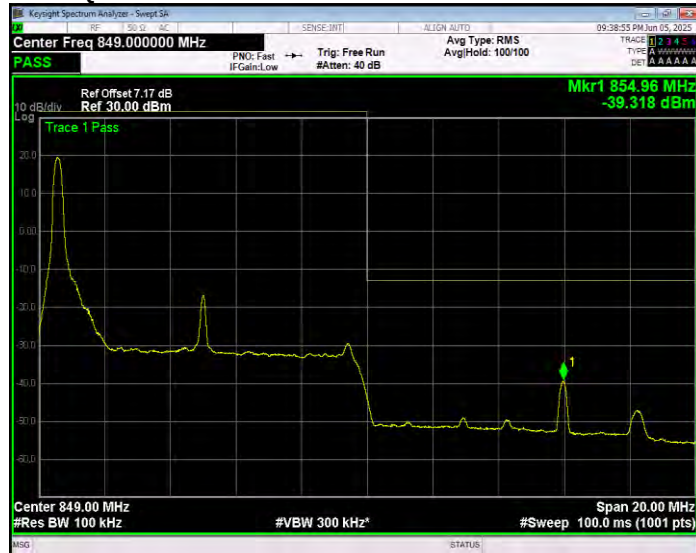
Band5 16QAM BW=10MHz Channel=20600 RB Size=1 Position=#Max Extended
