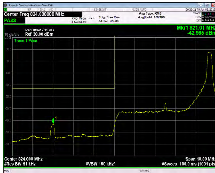
Band5 QPSK BW=5MHz Channel=20425 RB Size=25 Position=#0 Extended
