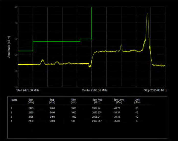
Band7 16QAM BW=20MHz Channel=20850 RB Size=100 Position=#0 Extended
