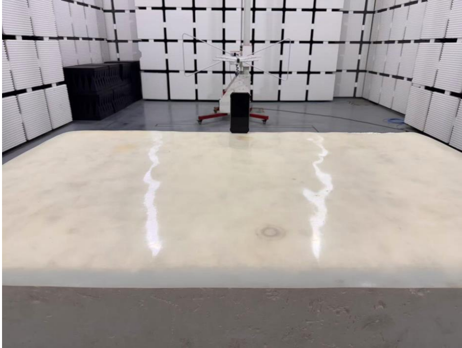
Set-up for Transmitter & Receiver Spurious Emissions, 30MHz to 1000MHz
