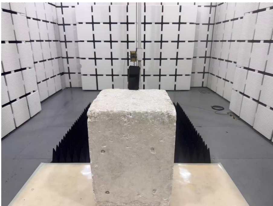
Set-up for Radiated Spurious Emission, Above 1GHz
