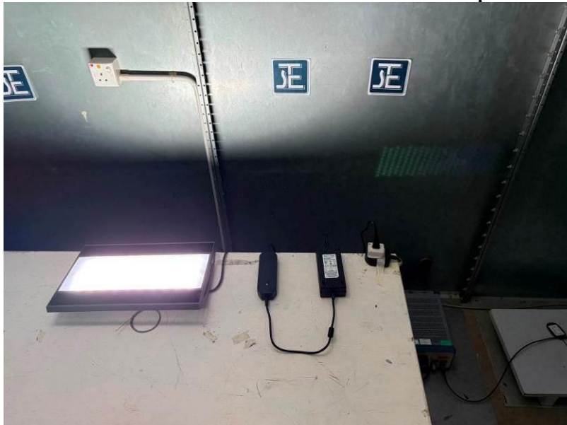
Measurement of Conducted Emission Test Set Up
