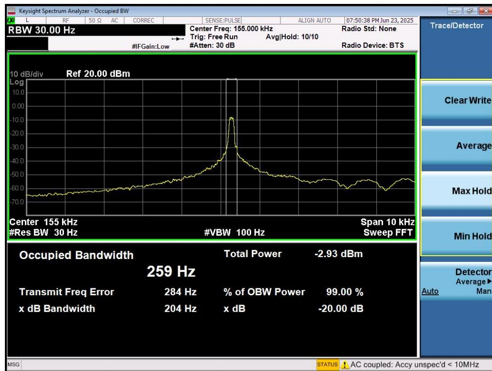
Note: Because the measured signal is CW-like, adjusting the RBW per C63.10 would not be practical since measurement bandwidth will always follow the RBW. The RBW is set to 30 Hz to perform the occupied bandwidth test.
