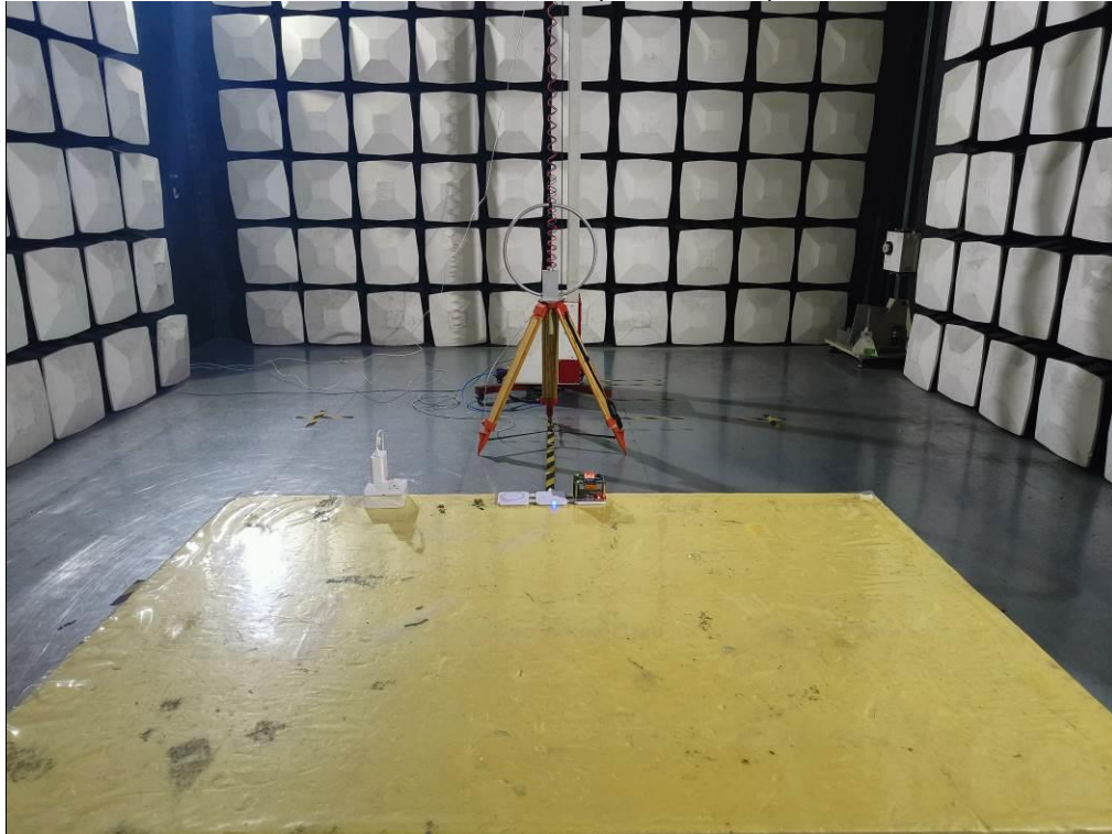
Test Photo Radiated emission (Below 30MHz)
