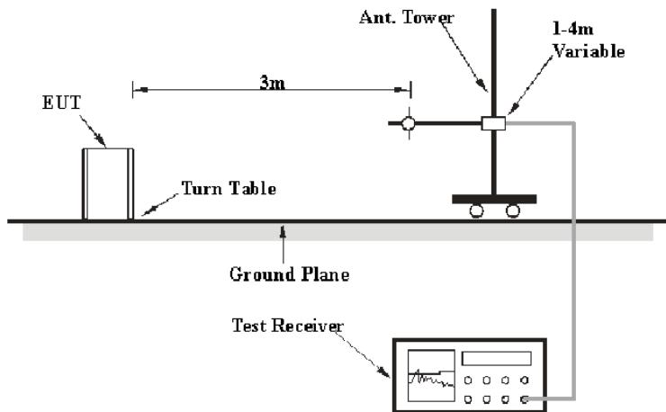
The radiated emission tests were performed in the 3-meter chamber test site, using the setup accordance with the ANSI C63.10-2013. The specification used was the FCC 15.209 limits.
