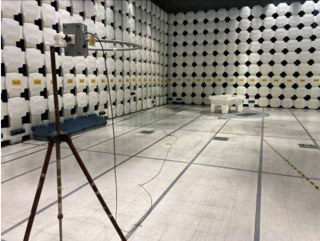
Config 2 – Wirelessly Charging IPG – 9kHz – 30MHz, FCC Part 18, Loop antenna on Z-Axis
