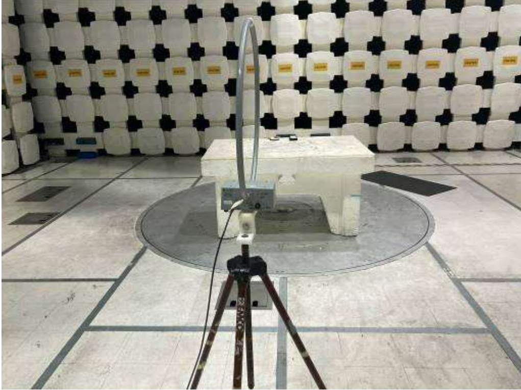
Config 2 – Wirelessly Charging IPG – 9kHz – 30MHz, 15.209, Loop antenna on Y-Axis
