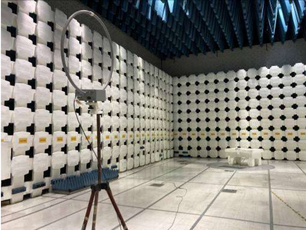
Config 2 – Wirelessly Charging IPG – 9kHz – 30MHz, FCC Part 18, Loop antenna on Y-Axis
