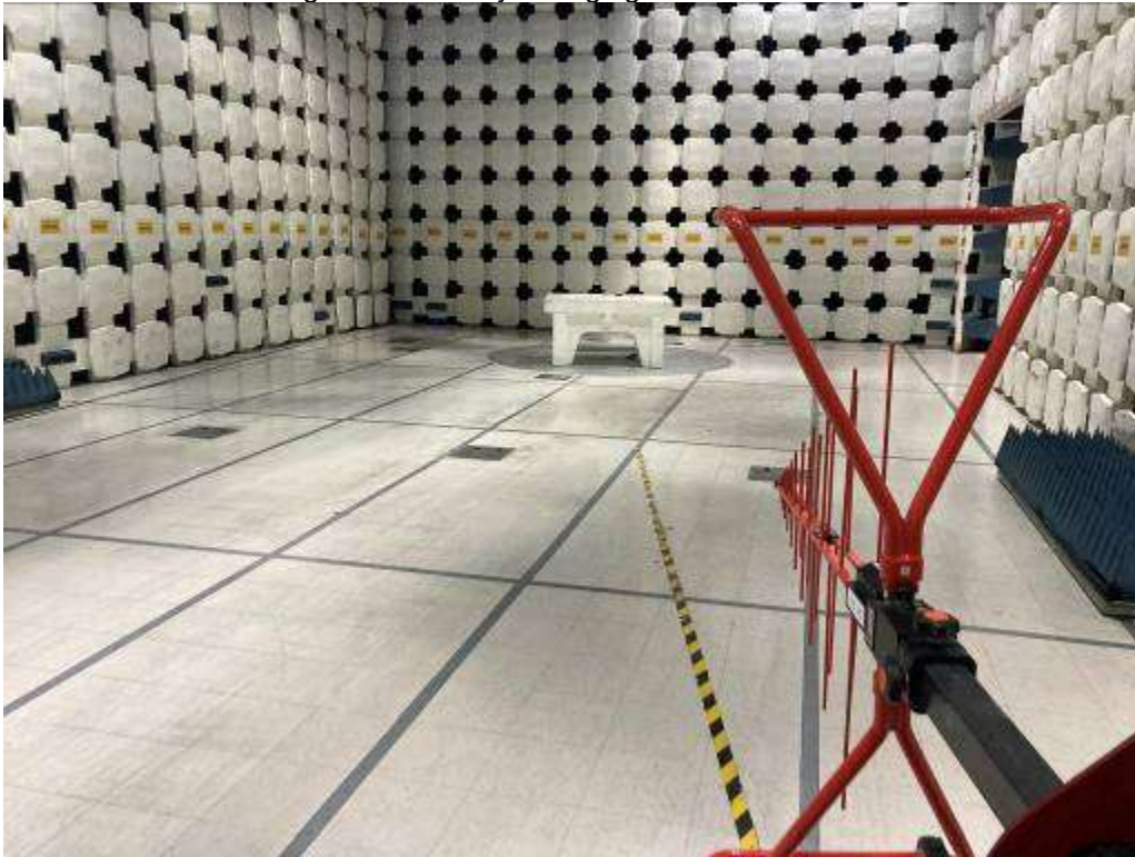
Config 2 – Wirelessly Charging IPG – 30-1000 MHz
