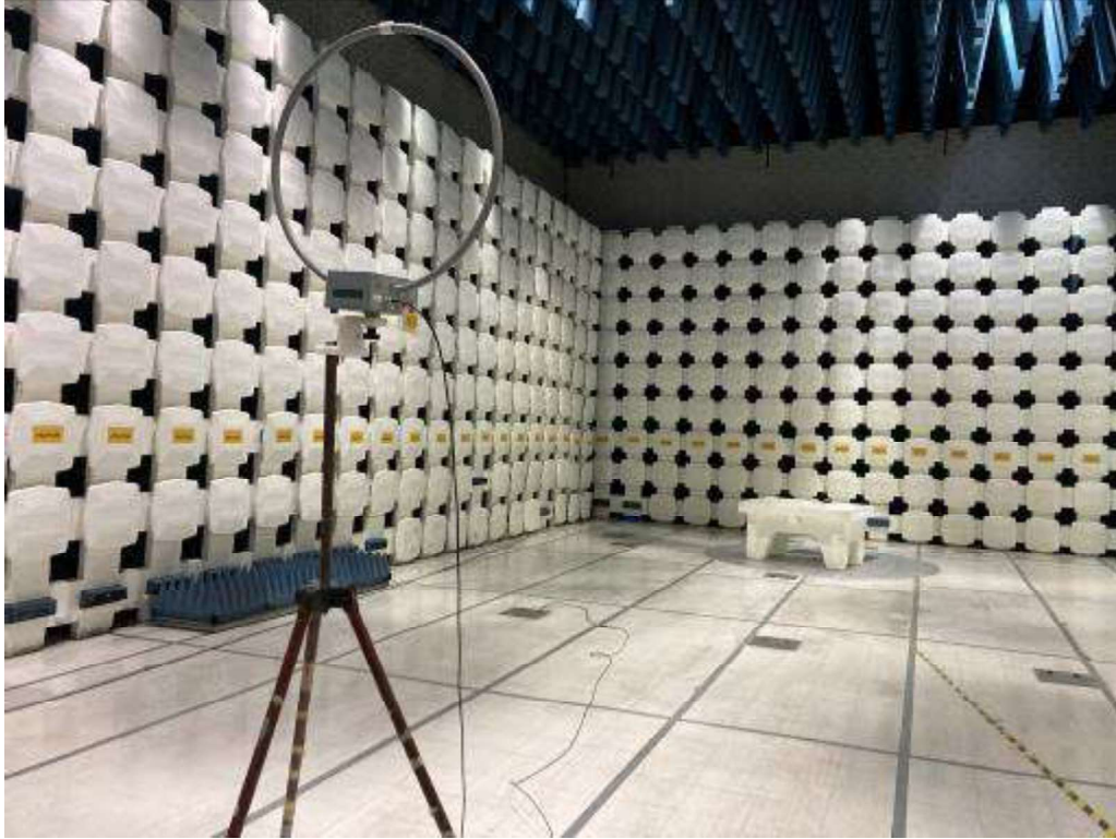
Config 2 – Wirelessly Charging IPG – 9kHz – 30MHz, FCC Part 18, Loop antenna on X-Axis
