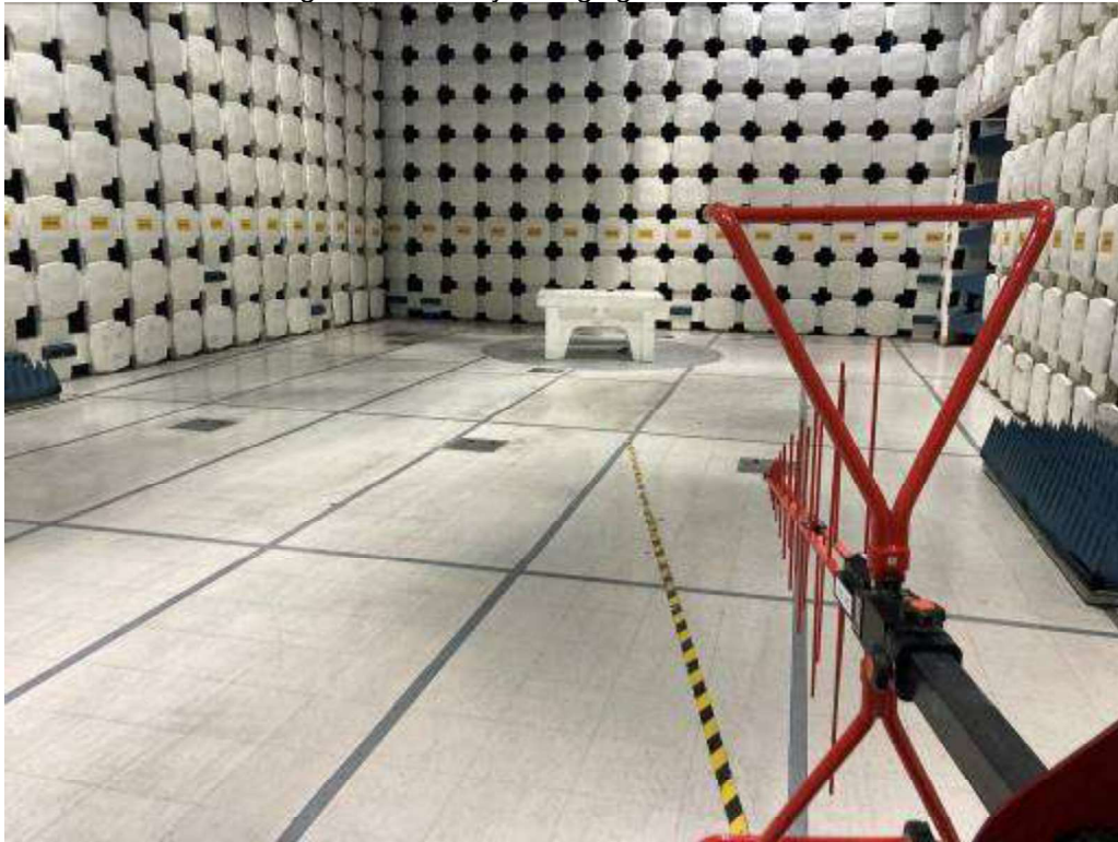
Config 2 – Wirelessly Charging IPG – 30-1000 MHz
