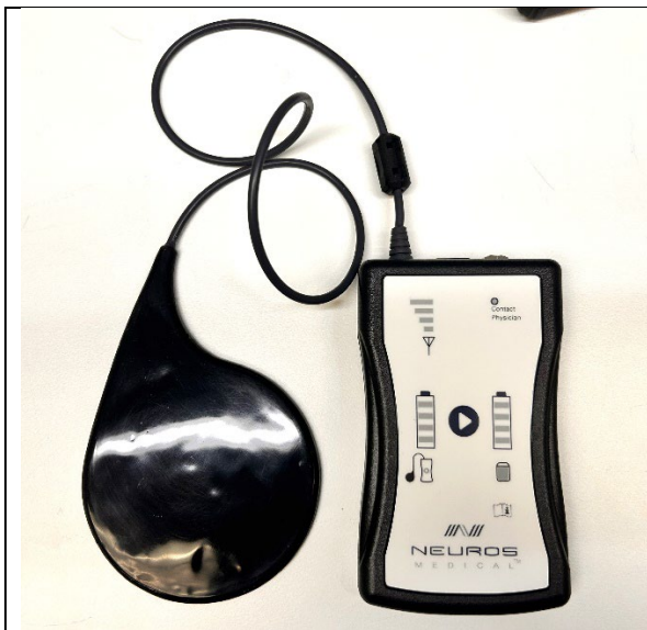
Battery Charger with Charging paddle, this is intended to show that the Charging Coil is contained in the charging paddle, which is permanently attached the chassis of the battery charger
