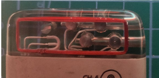
IPG Internal Photo, Charge Coil in Epoxy Header
