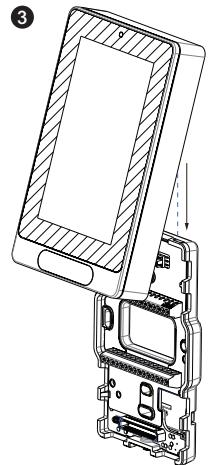
Gently push excess wiring back into the opening. Align the cover with the top of the base and slide it down.
