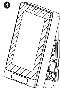
Once aligned with the top of the base, snap the cover into place from the bottom.
