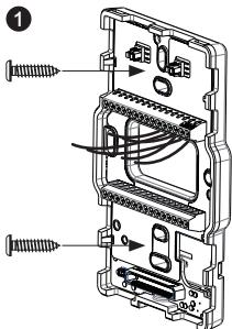
Use 2 screws to mount the base on the wall (maximum size #6, head diameter 6.9 mm (0.27 in)).
