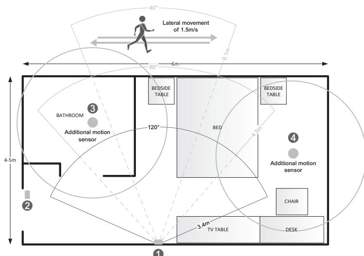
The internal Room Controller PIR sensor only detects lateral movement. It cannot detect movement when a person is moving toward it. It will not detect someone sitting on a chair and/or lying on the bed.
