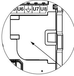
The Expansion Module Port allows you to insert one (1) module for CO<sub>2</sub> detection.\*
