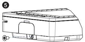
Install the security screw on the bottom of the unit using a square screwdriver.
