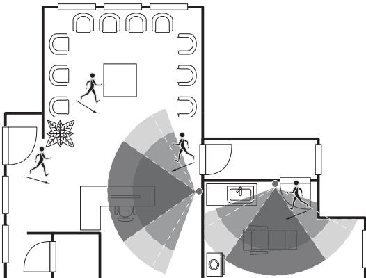
The examination room shows one Room Controller installed adjacent to the door. In this area of the room, occupant traffic is high and ensures the occupant will almost always cross the PIR detection path laterally and within the detection range.
