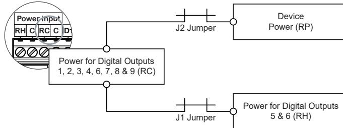
If a Relay Pack (or another isolated power supply) is used to power the Room Controller:
