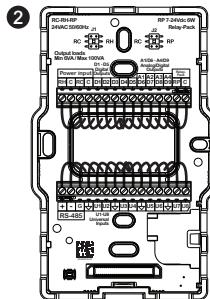
Strip each wire 6 mm (1/4 in) from the end, and use a flat screwdriver to secure wires to their terminals.
