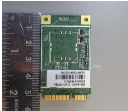
LTE Module rear view with Dimesions
