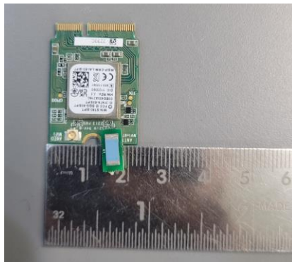
Wi-Fi Module with shield dimensional view
