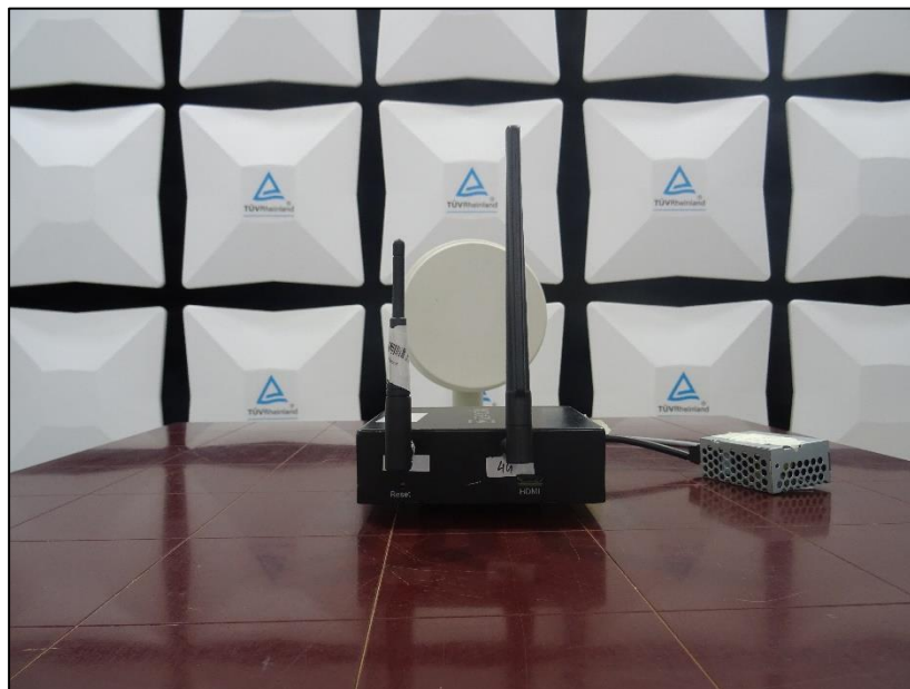
Above 1GHz Radiated Test Setup
