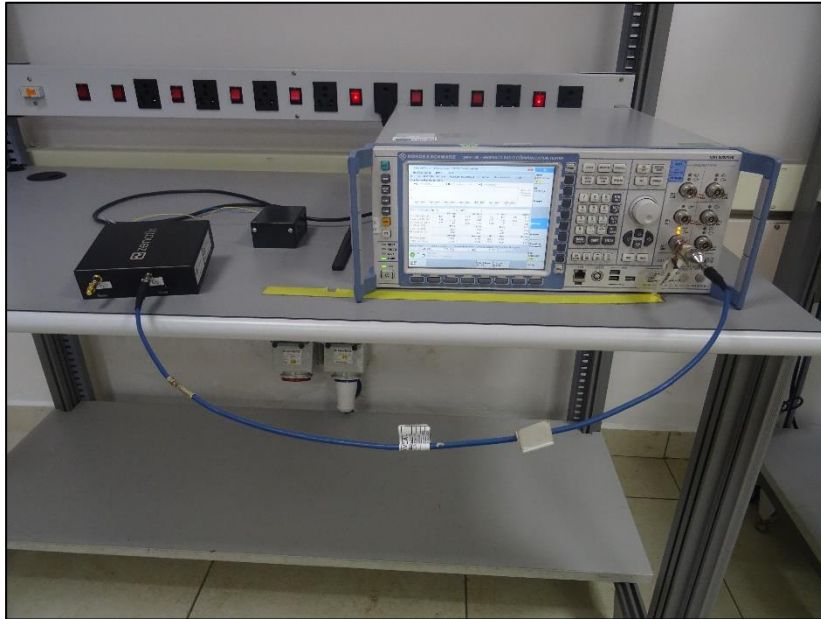
Conducted Test Setup
