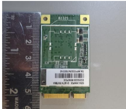
LTE Module rear view with Dimensions
