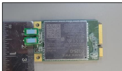
LTE Module Front View & Dimensions
