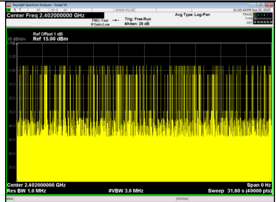
Number of Pulses in 31.6 seconds 8DPSK_3-DH5
