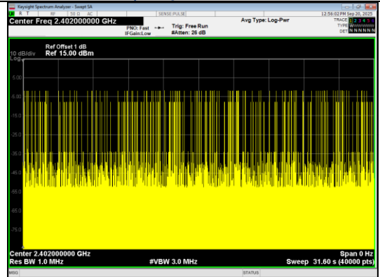
Number of Pulses in 31.6 seconds \pi/4 DQPSK_2-DH5
