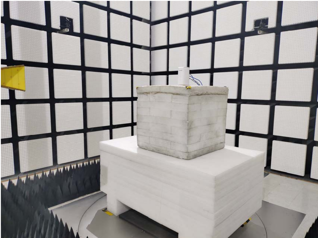
Radiated Emission Above 1GHz View-Adapter 1#
