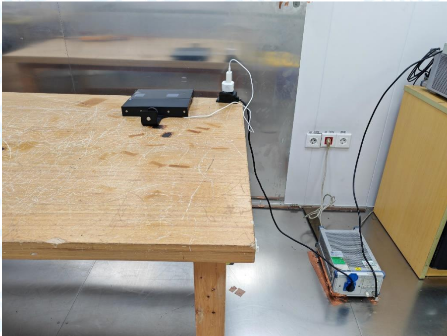
Photo of Setup for Radiated Emission (30MHz~1GHz)
