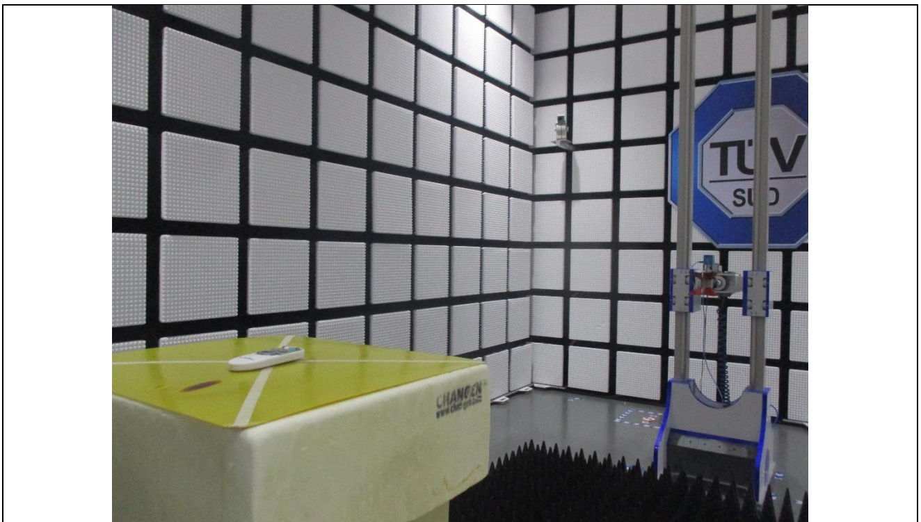
Radiated Emission test (1000MHz to 18000MHz)
