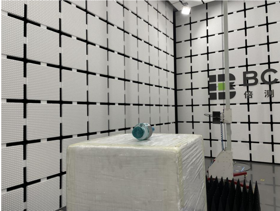
Spurious Emission Test Setup (Above 1GHz)
