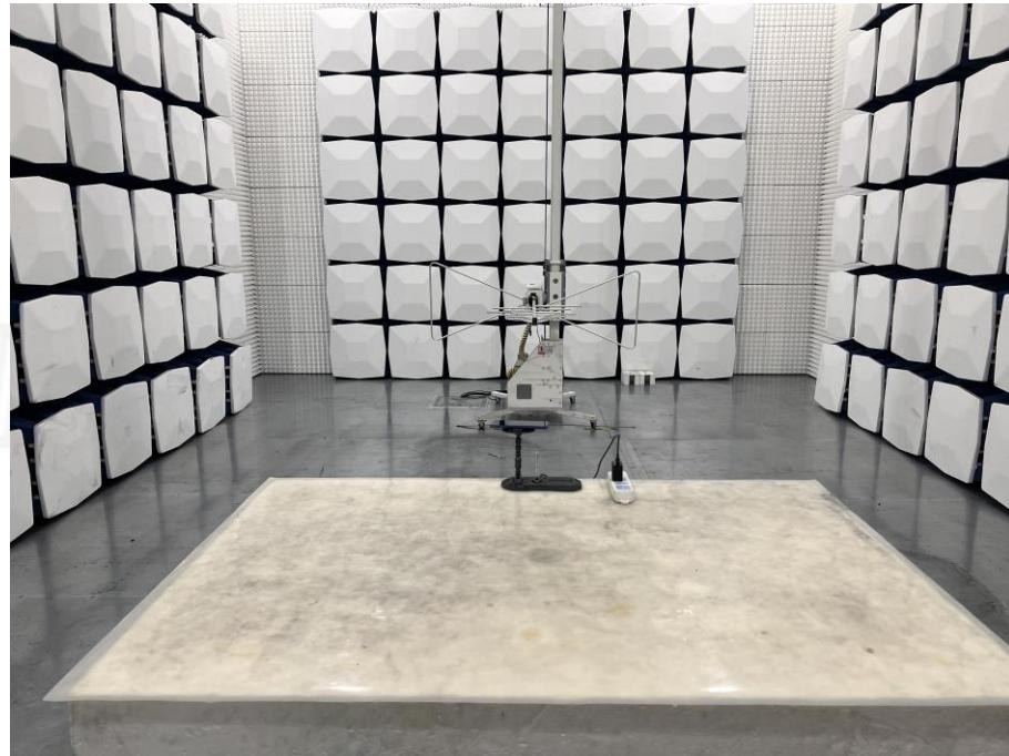
Radiated band emission (9KHz-30MHz):
