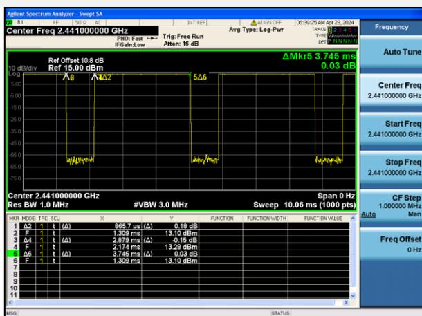
Note: The Bluetooth duty cycle is 76.88% as following figure, according to 2016 Oct. TCB workshop for Bluetooth SAR scaling need further consideration and the maximum duty cycle is 100%, therefore the actual duty cycle will be scaled up to 100% for Bluetooth reported SAR calculation.
