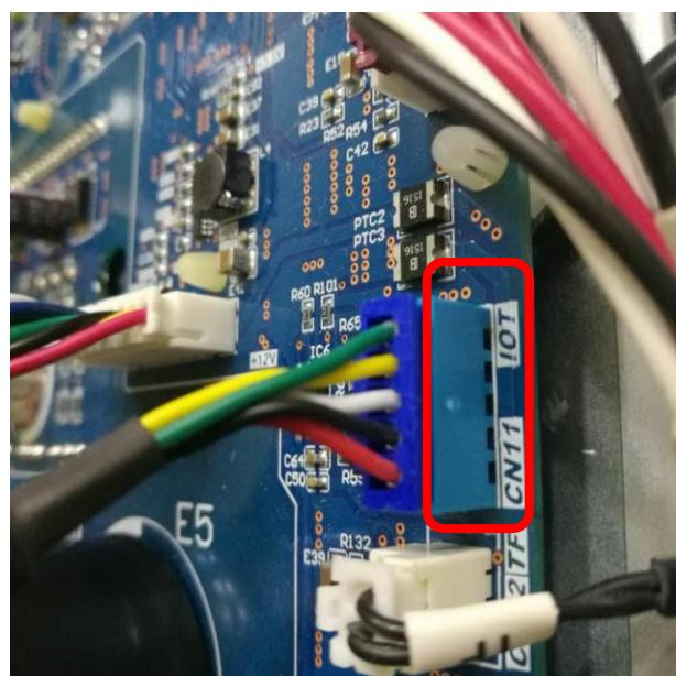
Power ON the condensing unit and check if the IoT device is working properly. The normal working state of IoT device should be the blue LED (No.1) is blinking with other LEDs light OFF.
