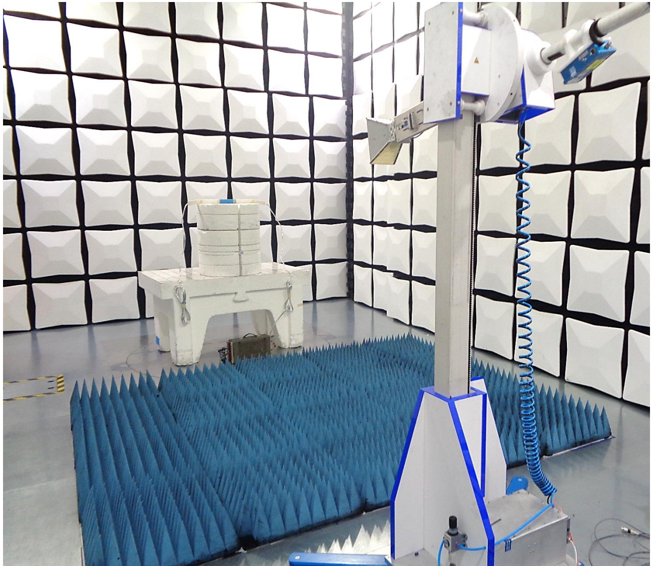
Figure 2: Test Setup for Radiated Emissions 1GHz to 18GHz
