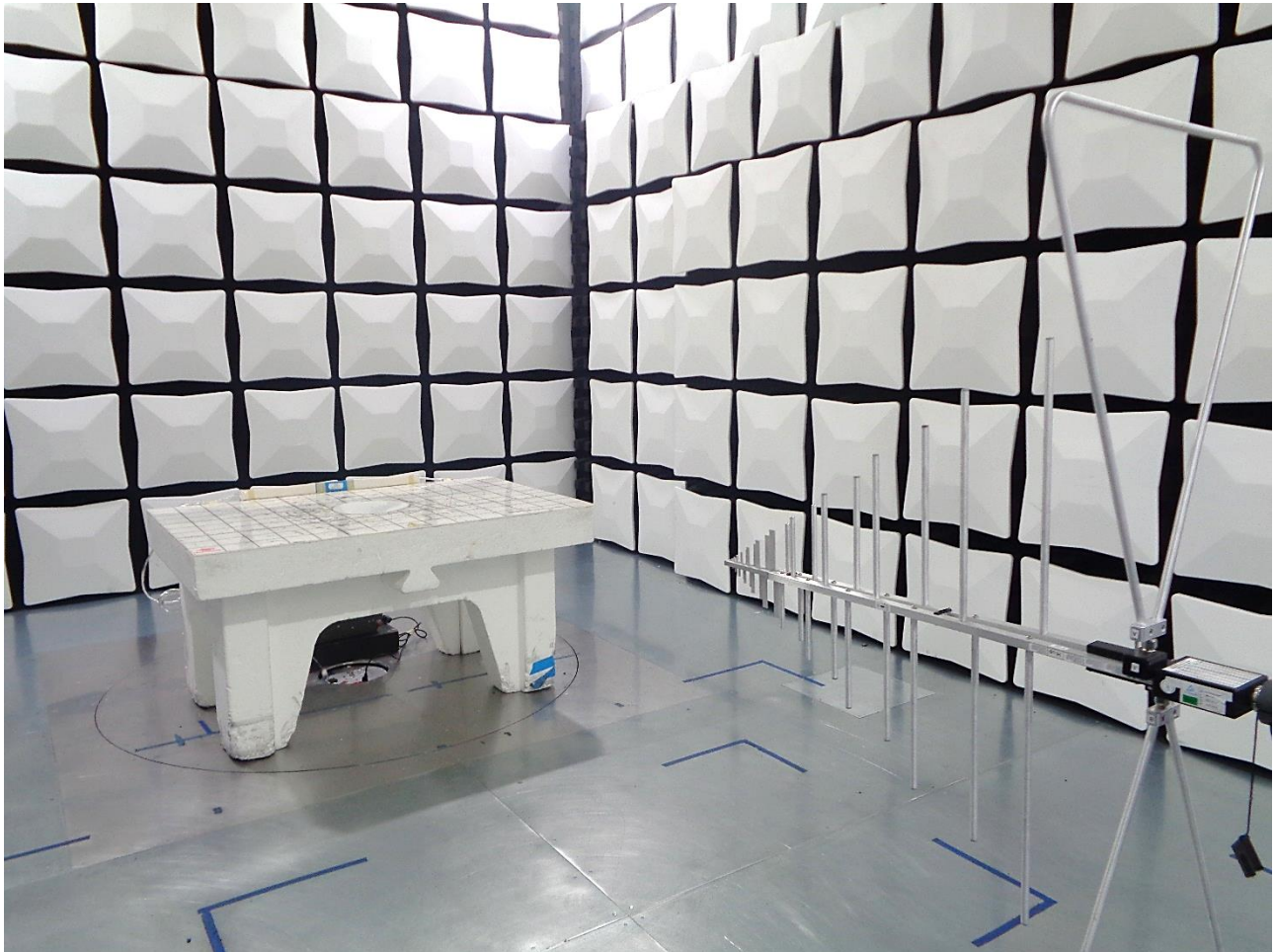
Figure 1: Test Setup for Radiated Emissions 30MHz to 1000MHz
