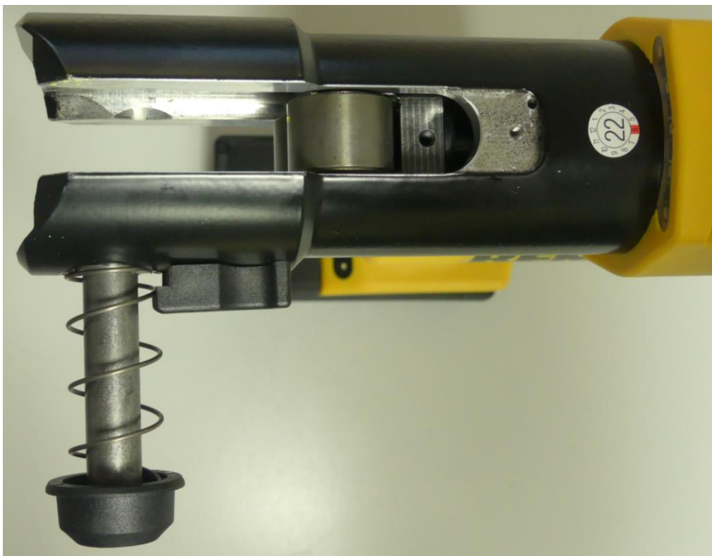
tong retaining bolt open, without protection for press rolls Eurofins Electric & Electronic Product Testing AG
