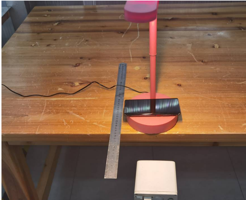
Test Position A-15cm from the edge of EUT to the geometric center of the probe
