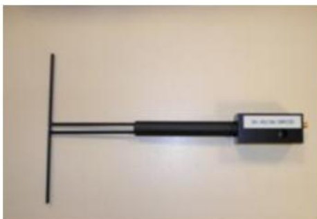
Figure 1 – Satimo COMOSAR Validation Dipole
