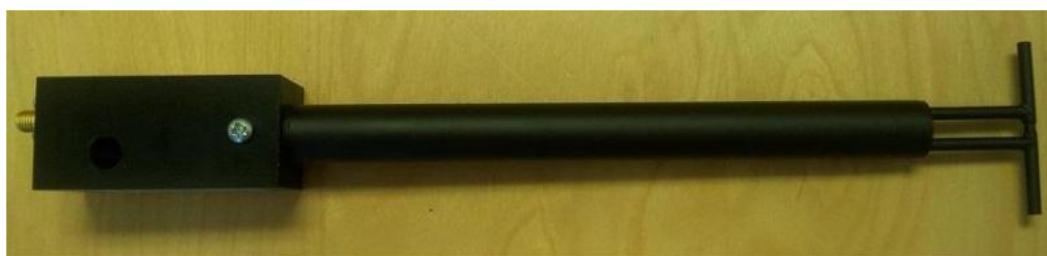
Figure 1 – MVG COMOSAR Validation Dipole
