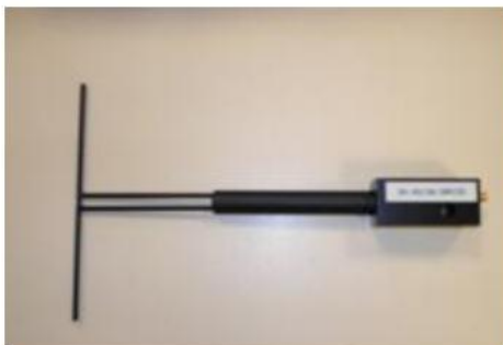
Figure 1 – Satimo COMOSAR Validation Dipole
