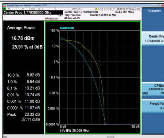
Band66-1.4MHz-QPSK-132665-6-0-High-10.21-<=13-PASS
